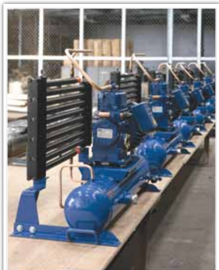
Tube-in-Tube Water Cooled Condensing Unit manufactured and assembled in the ITC's factory.
